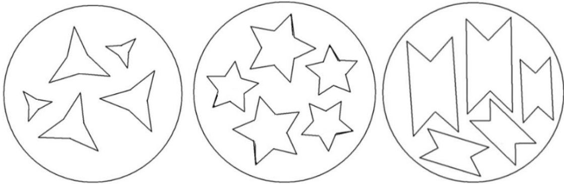
Figure 1. Illustrations to the optimized packings of non-convex polygons in a circular container.
